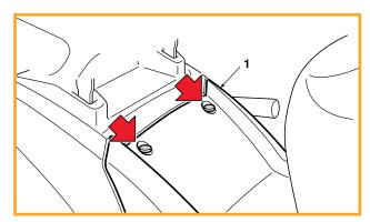
The brake adjustment spring can be accessed by removing the inspection hatch (1).
